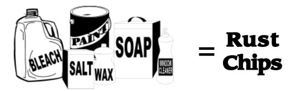
Contaminants in combustion air can lead to premature heater failure. Vapors from bleaches, soaps, waxes, salts, etc. are drawn into the combustion chamber with the make-up air and, once fired, mix with water vapor in the gases to form extremely corrosive hydrochloric or hydrofluoric acid and other corrosive by-products.
